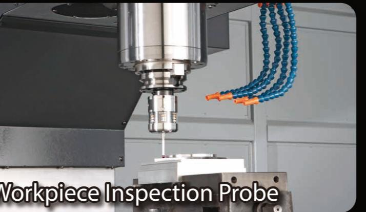
Workpiece Inspection Probe
